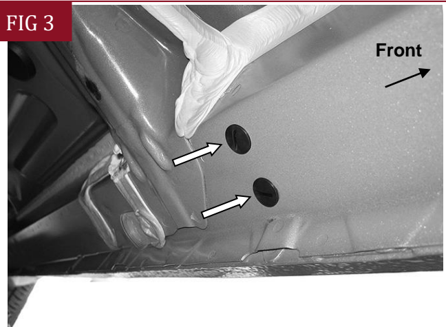
(Fig 3) Driver/Left center mounting location
