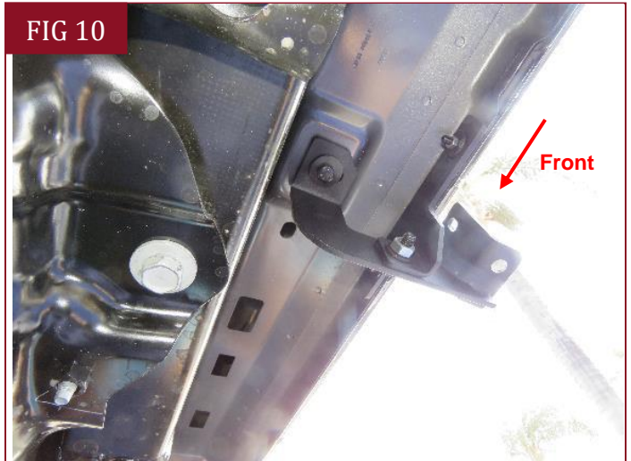
(Fig 10) Attach Passenger/Right Center Bracket and Passenger/Right Center Support Bracket to the center location
