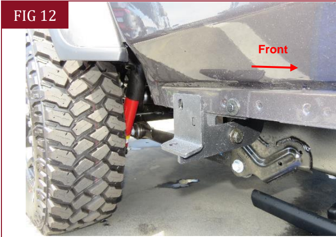
(Fig 12) Attach Passenger/Right Rear Bracket and Passenger/Right Rear Support Bracket to the rear location
