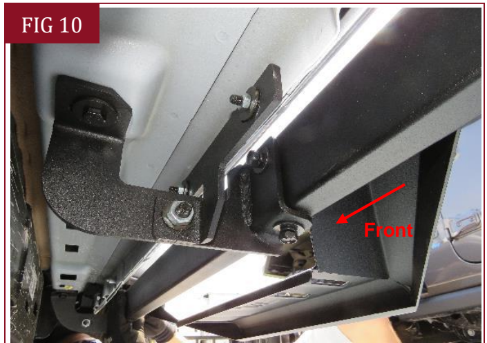
(Fig 10) Passenger/Right rear mounting bracket and support bracket attached.
