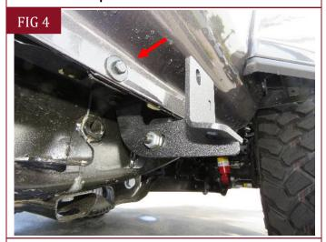
(Fig 4) Insert Bolts from the outside of the pinch weld.
