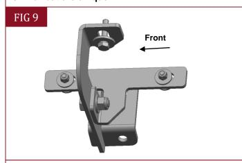
(Fig 9) Attach Passenger/Right Center Bracket and (1) Passenger/Right Center/Rear Support Bracket (#2) to the center location
