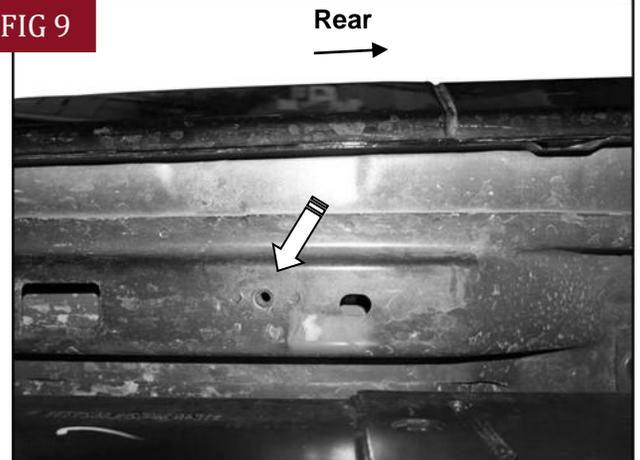
(Fig 9) Driver/Left rear mounting location (Models with threaded insert shown)
