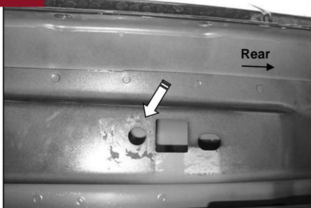
(Fig 8) Driver/Left rear mounting location (Models with open mounting location shown)
