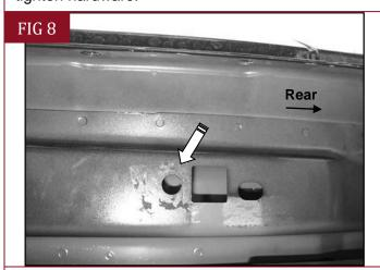
(Fig 8) Driver/Left rear mounting location (Models with open mounting location shown)
