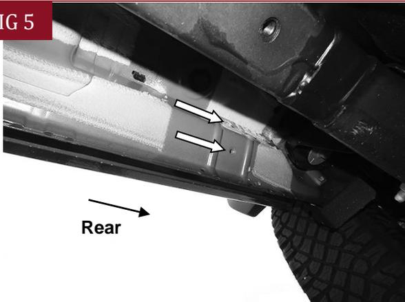
(Fig 5) Passenger/Right rear mounting location
