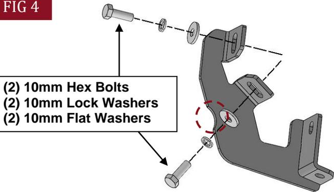
(Fig 4) Attach (1) Passenger/Right Center Mounting Bracket to the center location. **Note: A Bigger Notch on the rear of the Center Brackets**
