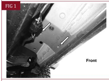
(Fig 1) Passenger/Right front mounting location
