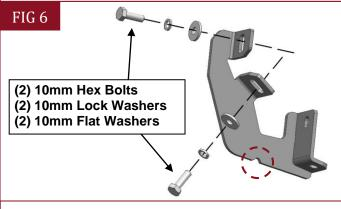
(Fig 6) Attach (1) Passenger/Right Rear Mounting Bracket to the Rear location. Note: A Smaller Notch on the bottom of the Rear Brackets
