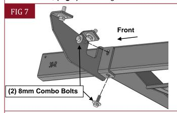
(Fig 7) Attach the Passenger/Right Running Board to the Mounting Brackets
