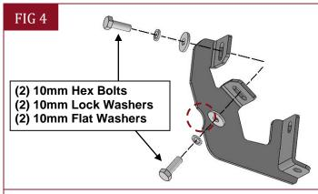
(Fig 4) Attach (1) Passenger/Right Center Mounting Bracket to the center location. Note: A Bigger Notch on the rear of the Center Brackets
