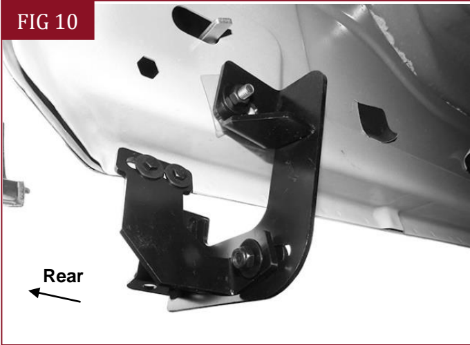
(Fig 10) Driver/left Side Step attached to Rear Brackets
