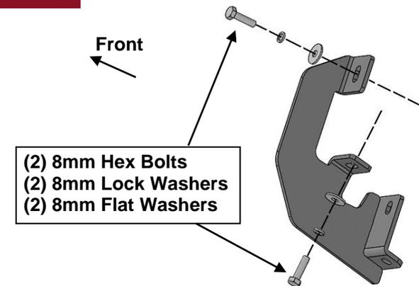
**(Fig 3) Attach (1) Mounting Bracket to the Passenger/Right front location**
