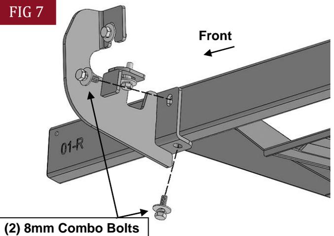
(Fig 7) Attach the Passenger/Right DS7 Running Board to the Mounting Brackets
