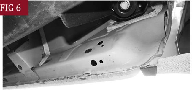
(Fig 6) Remove rubber plugs from the Passenger/Right rear mounting location
