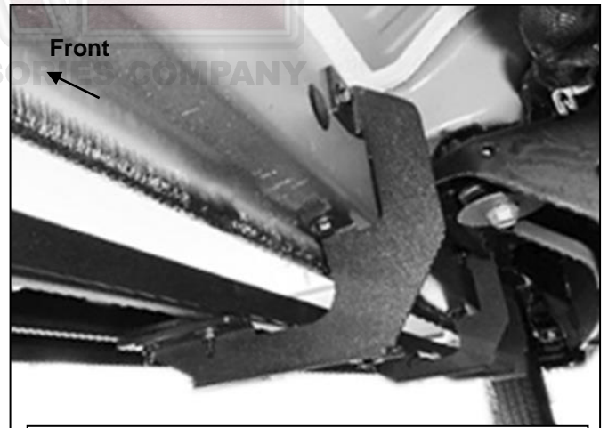
(Fig 12) Passenger/right #2 Bracket installation
