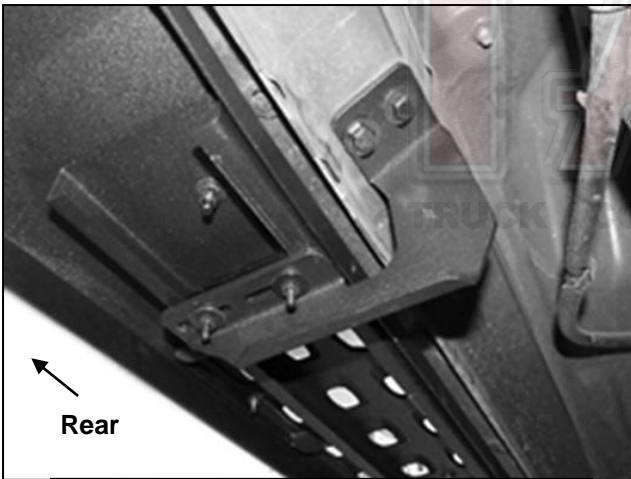
(Fig 12) Driver/left rear Bracket installed
