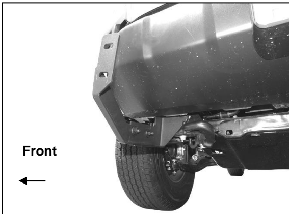
(Fig 8) Passenger/right Bull Bar Bracket attached to inside of Frame Bracket (pictured without air dam)
