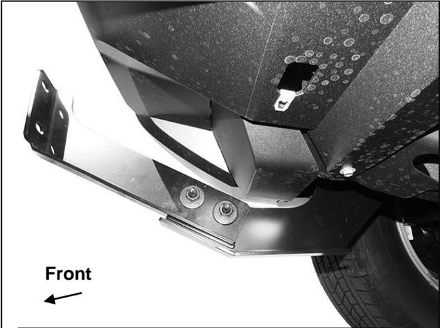
(Fig 9) Passenger/right Bull Bar Bracket attached to Frame Mounting Bracket
