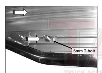
(Fig 17) Slide (3) T-Bolts into each channel
