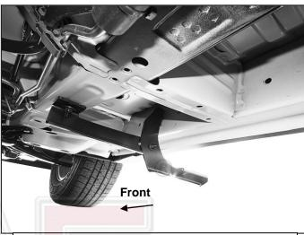
(Fig 7) Passenger/Right Front Brackets attached
