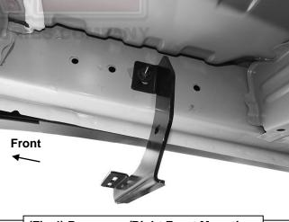
(Fig 4) Passenger/Right Front Mounting Bracket attached to inner body panel
