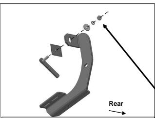
(Fig 14) Attach Passenger/Right Rear Mounting Bracket to Bolt Plate in body panel
