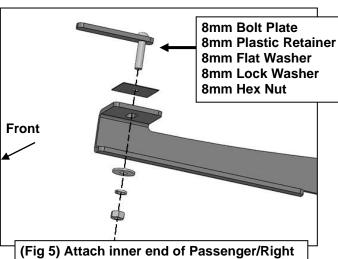
Front Support Bracket to Bolt Plate in frame
