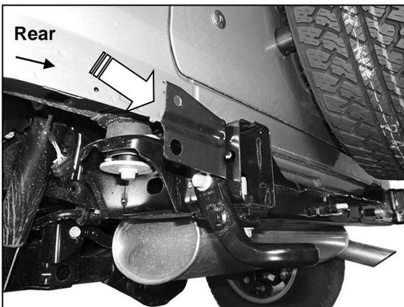
(Fig 5) Remove inner bumper bracket and tow hook from side of frame
