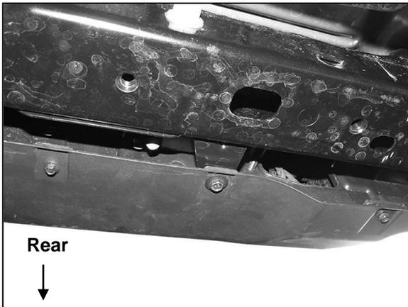
(Fig 1) Remove (2) hex bolts (if equipped) attaching bottom of bumper to cross member
