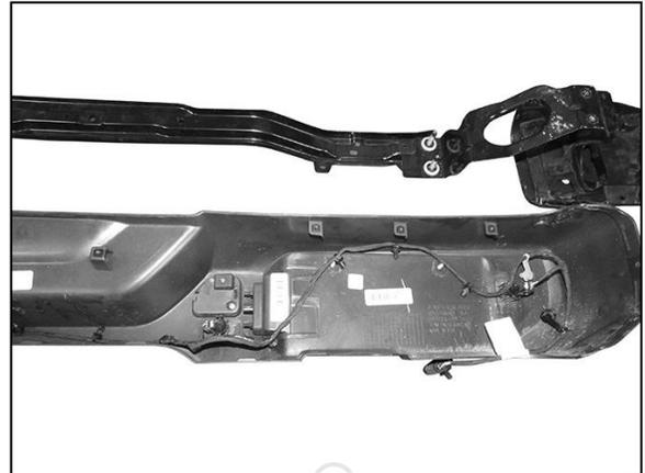
(Fig 7) Disassemble bumper, if necessary, to remove sensors and wiring harness
