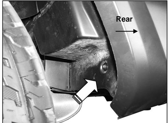
(Fig 2) Remove plastic cover from back of bumper (arrow-driver/left side pictured)
