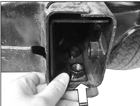
(Fig 10) Insert U-Bracket into end of passenger side frame. Line up weld nuts with holes
