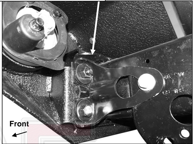
(Fig 15) Bumper installed on JL. Driver/left outer installation pictured from behind Bumper
