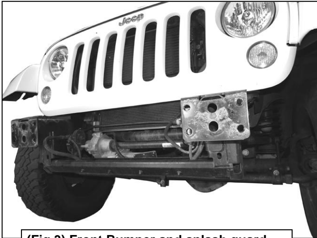
(Fig 3) Front Bumper and splash guard removed from 2007-18 JK model pictured
