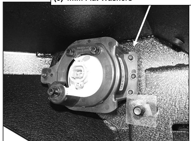
(Fig 13B) Attach offset style fog light directly to mounting plates. Driver/left side pictured
