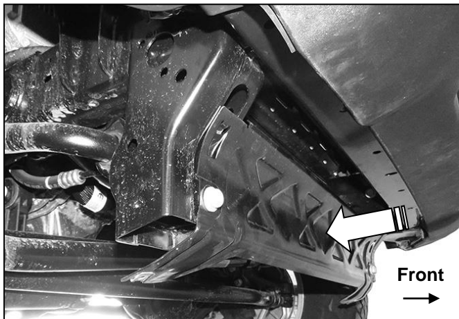
(Fig 1) Remove splash guard and bracket (arrow)
