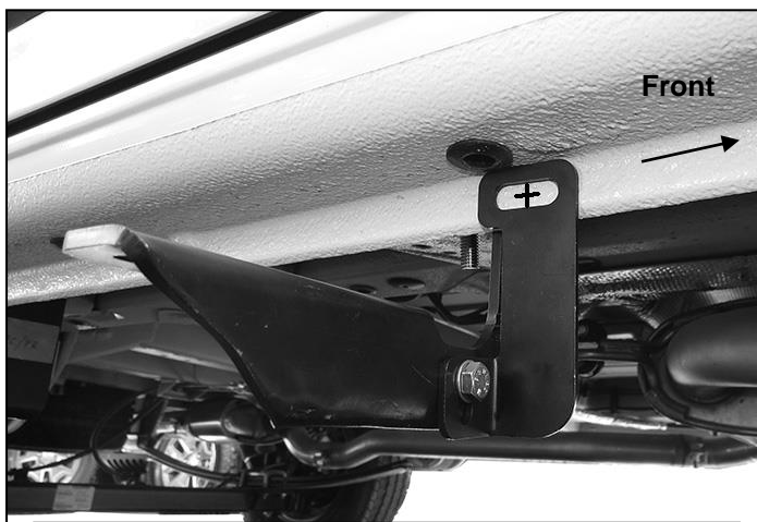
(Fig 20) Passenger side center Bracket installed
