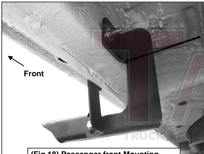
(Fig 18) Passenger front Mounting Bracket and Support Bracket installed
