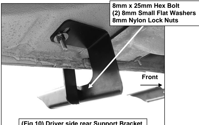
(Fig 10) Driver side rear Support Bracket
