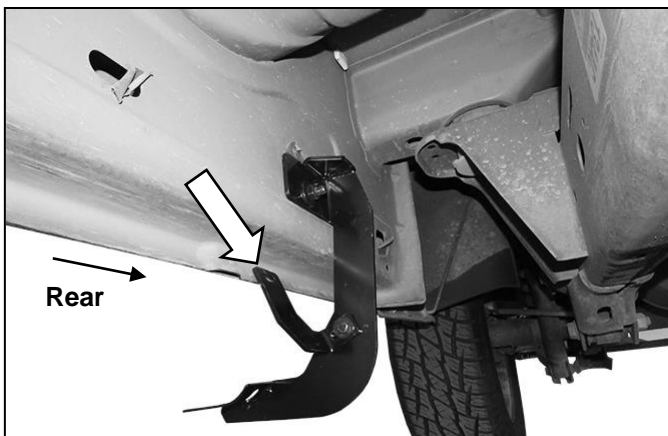
(Fig 10) Attach the Passenger/Right Rear Support Bracket to the Rear Mounting Bracket. Mark the location of the upper slot in the Support Bracket on the pinch trim for drilling. Use a 1/4inch drill bit, (drill bit not included)
