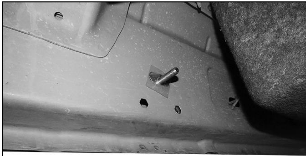
(Fig 6) Insert (1) 10mm Bolt/Nut Plate into the upper slot and line the threaded nut up to the rear hex hole, Thread (1) 10mm Plastic Retainer over the threads to hold it in place
