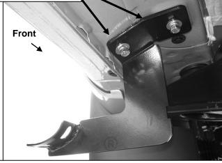
(Fig 2) Driver side front mounting location pictured
