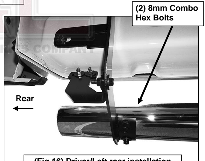
(Fig 16) Driver/Left rear installation
