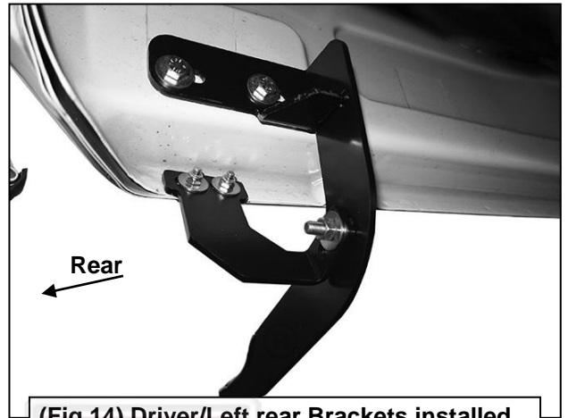
(Fig 14) Driver/Left rear Brackets installed
