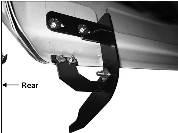
(Fig 16) Driver/Left rear Mounting Bracket assembly
