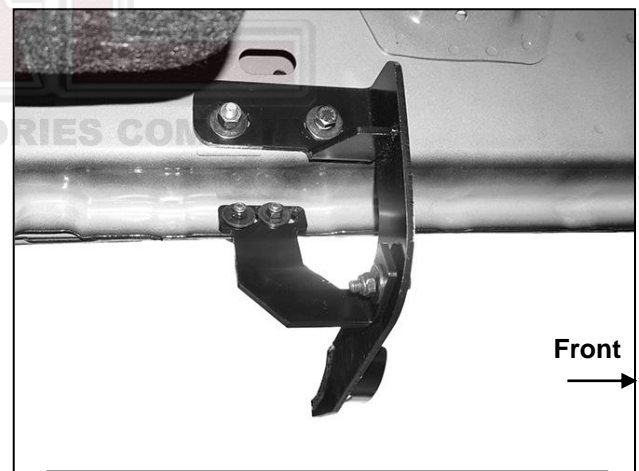
(Fig 14) Attach Driver/Left center Bracket
