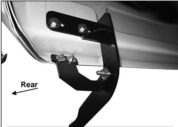
(Fig 16) Driver/Left rear Brackets installed
