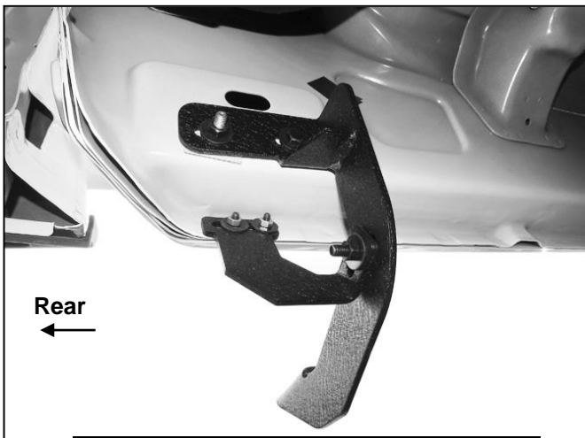
(Fig 16) Driver/left side rear Brackets attached to body panel and pinch weld
