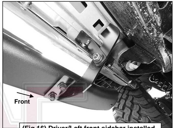
(Fig 16) Driver/Left front sidebar installed
