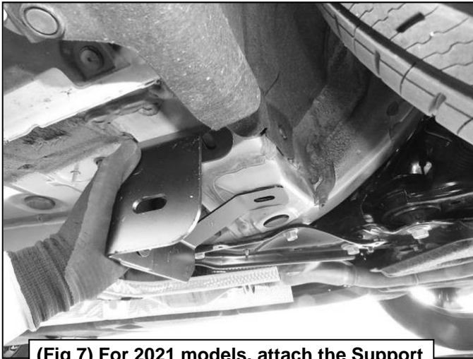
(Fig 7) For 2021 models, attach the Support Bracket to the Mounting Bracket. Mark the upper slot in the Support Bracket
