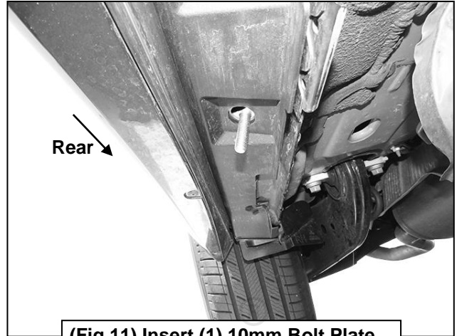
(Fig 11) Insert (1) 10mm Bolt Plate into the outer hole in the floor panel
