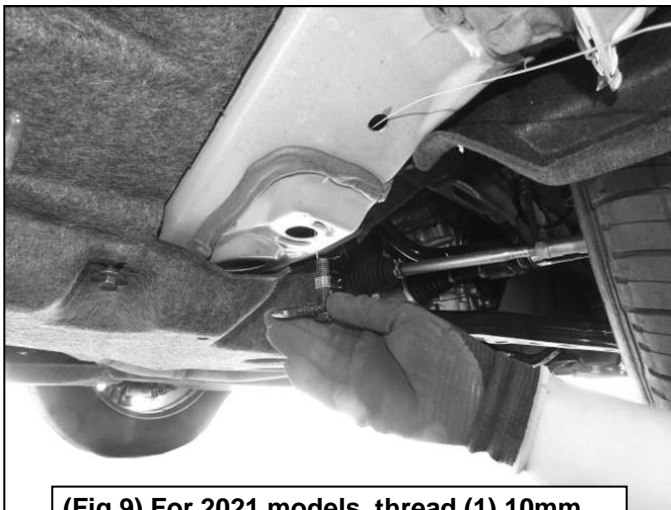
(Fig 9) For 2021 models, thread (1) 10mm Bolt Plate into the Fish Wire. Guide the end of the Fish Wire into the large hole and out the drilled hole. Pull the Bolt Plate through
