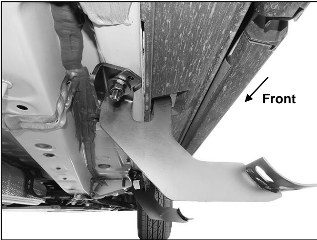
(Fig 17) Passenger/Right Center Bracket installed
