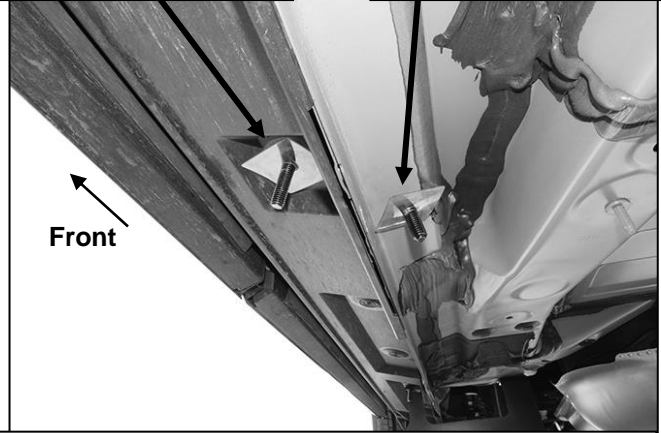
(Fig 16) Insert 8mm Bolt Plate and 10mm L-Shaped Bolt into the Passenger/Right Center mounting holes
