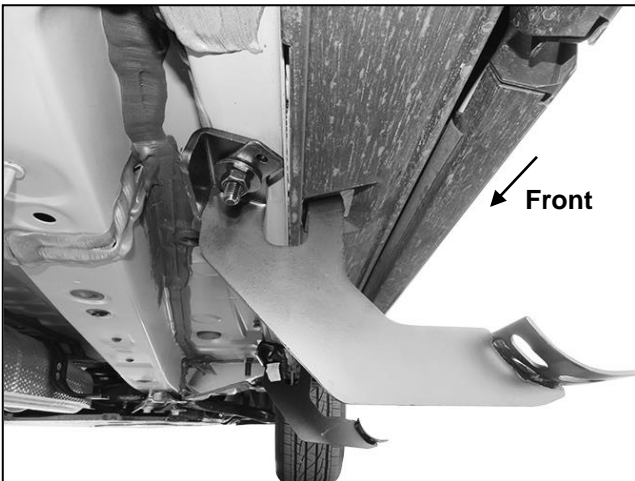
(Fig 17) Passenger/Right Center Bracket installed
