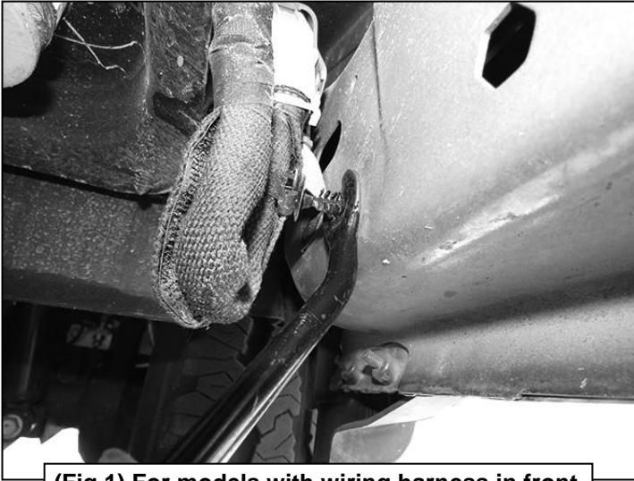
(Fig 1) For models with wiring harness in front mounting location, use a pry tool to remove the pin and loosen the wiring. Push out of the way for Mounting Bracket installation.
