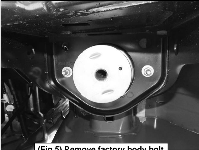
(Fig 5) Remove factory body bolt
