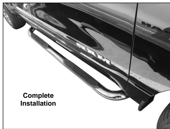
(Fig 12) Driver/left Front Brackets and Sidebar installed
