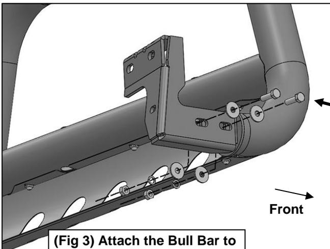
(Fig 3) Attach the Bull Bar to the (2) Mounting Brackets
