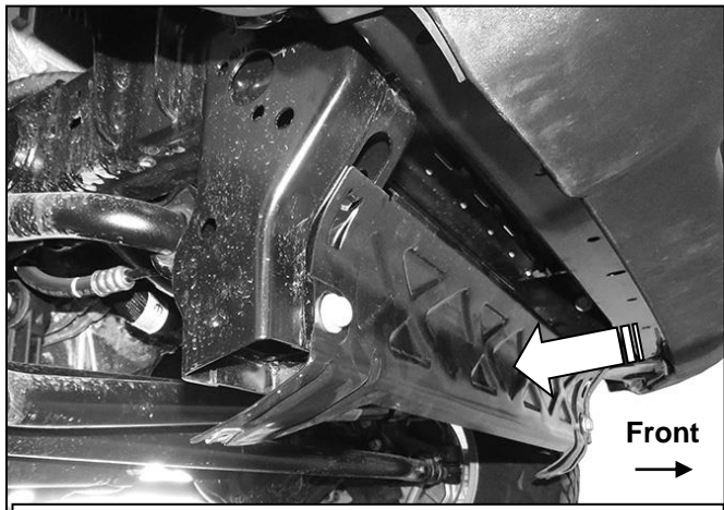
(Fig 1) Remove splash guard and bracket (arrow)
