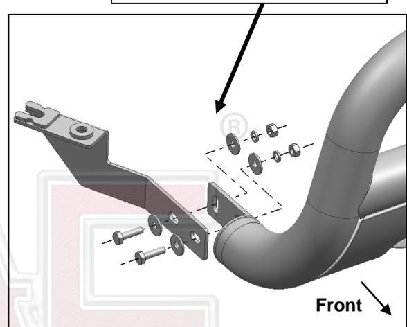
**(Fig 5) Attach Bull Bar to inside of Mounting Brackets (passenger/right side illustrated)**
