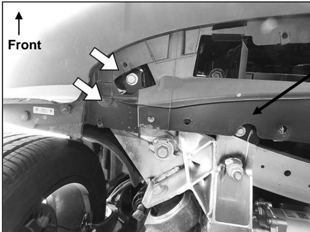
Remove splash guard from bottom of bumper
