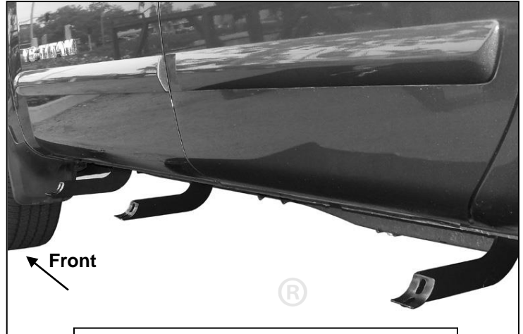
(Fig 4) Driver side Brackets installed. Note all cradles face back of vehicle
