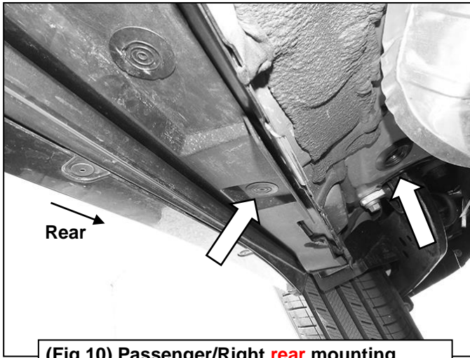
(Fig 10) Passenger/Right rear mounting location, Remove plastic plugs from holes
