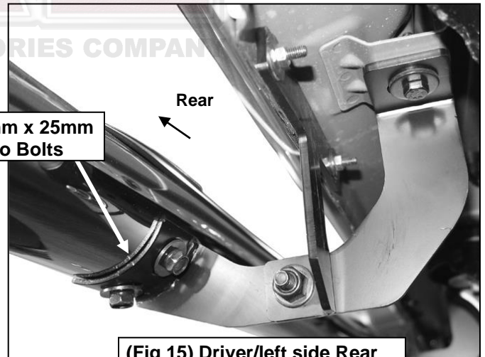
(Fig 15) Driver/left side Rear Brackets attached to Sidebar
