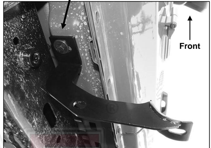
(Fig 4) Driver/left front Mounting Bracket installed
