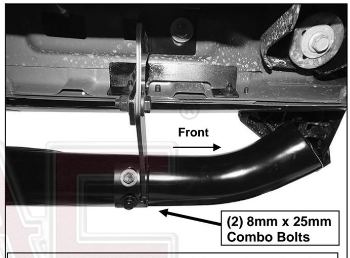
(Fig 16) Attach driver/left Sidebar to front Bracket
