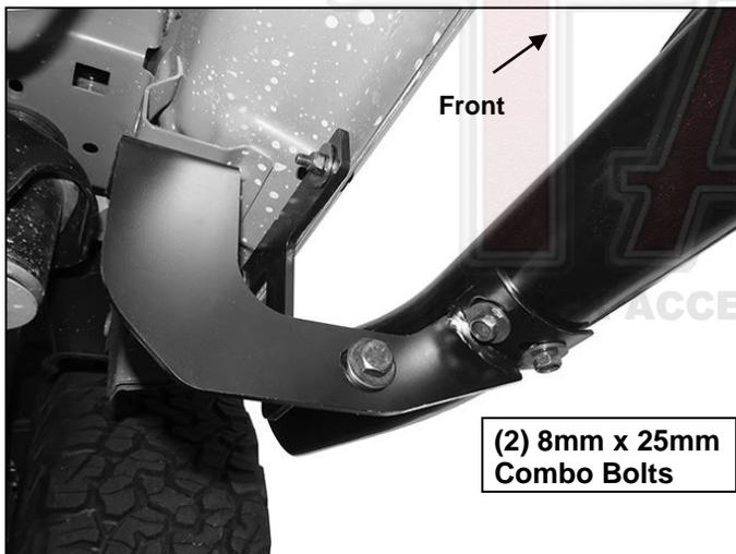
(Fig 17) Driver/left Sidebar attached to rear Bracket
