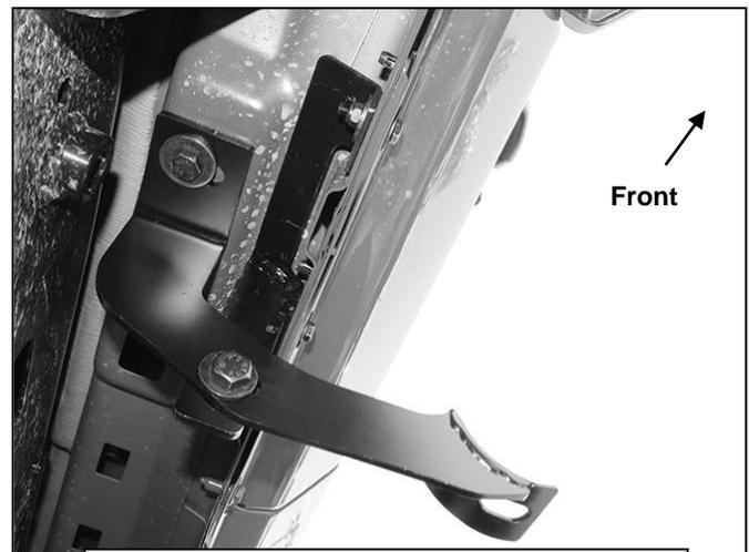
(Fig 6) Driver/left front Brackets installed
