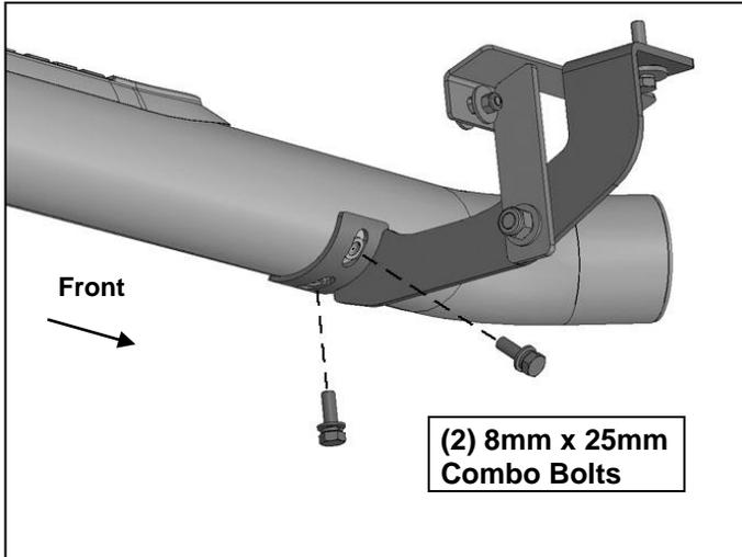
(Fig 15) Attach driver/left Sidebar to front Bracket
