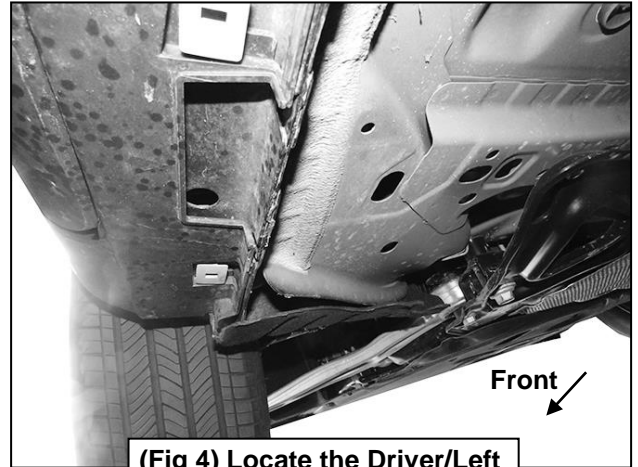
(Fig 4) Locate the Driver/Left front mounting location
