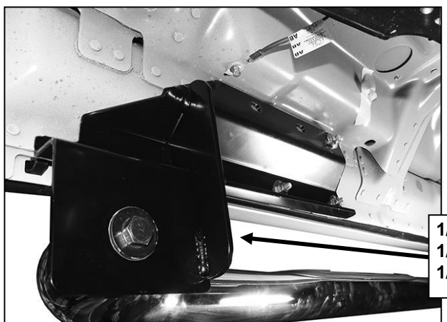
(Fig 5) Passenger side front Bracket installation
