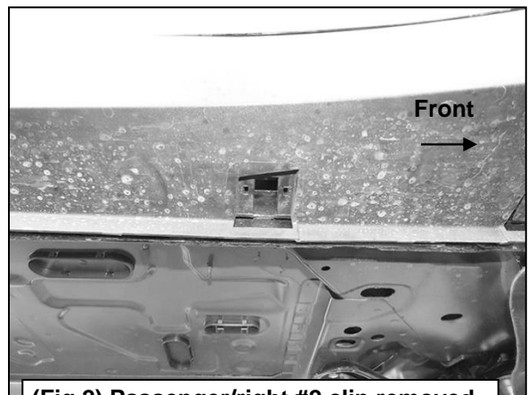
(Fig 2) Passenger/right #2 clip removed
