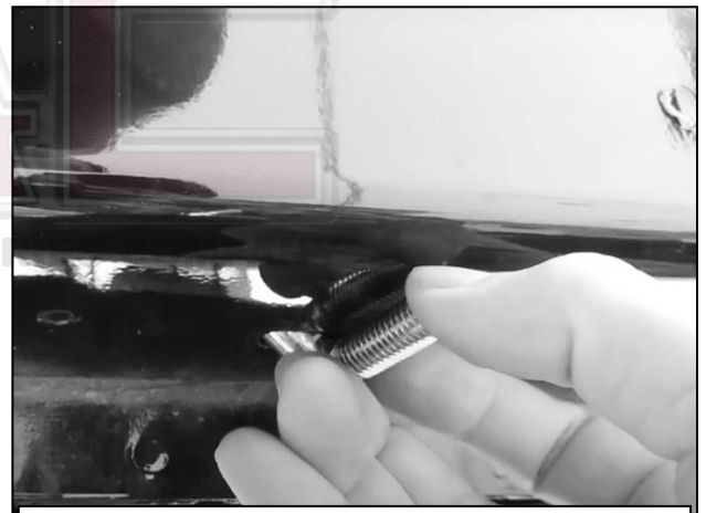
(Fig 6) Insert the bend on the tail into the slot, keeping the threads pointed outwards
