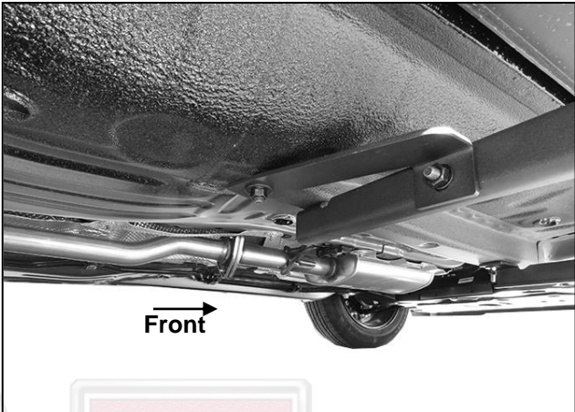
(Fig 10) Passenger/Right Center Support Bracket attached to the Bolt Plate and Mounting Bracket
