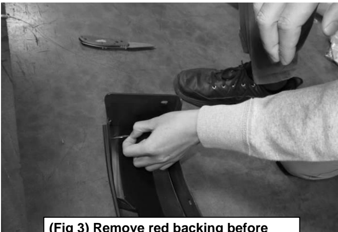
(Fig 3) Remove red backing before applying rubber trim to prevent waste of adhesion promoter
