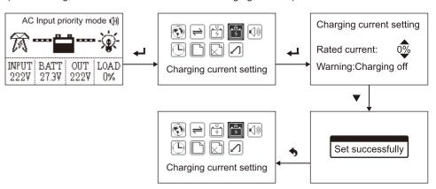
**Note**: The rated current is 0%-100% of the maximum charging current.
