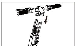
4. Align the scooter's head with the stem.
