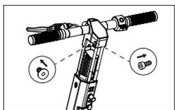
5. Tighten the screws to secure the scooter's head with the provided tool.
