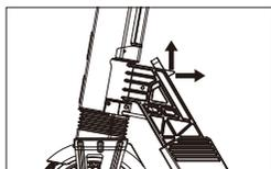
2. Pull up the lock in the middle to release the latch.
