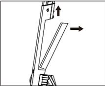
2. Hold and pull the upper part of the battery pack outwards while holding up the battery release button.
