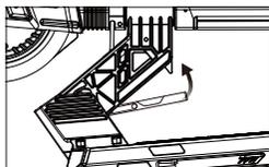
4. Pull up the latch to secure it with the lock until a "click" sound is heard.
