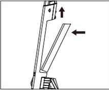
2. Pull up the battery release button while pushing the upper part of the battery pack into the stem.
