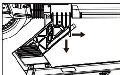
1. Pull up the lock in the middle to release the latch.
