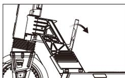
3. Press down the latch to completely fold up the stem.
