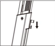
3. Push down the battery release button to secure the battery pack into the stem.
