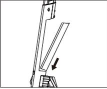
1. Align the bottom of the battery with the stem.
