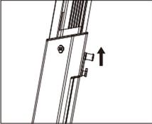
1. Pull up the battery release button on the stem.
