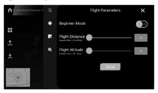
Tap to set the maximum flight distance and flight altitude. Beginner mode with preset flight parameters is recommended for beginners.
