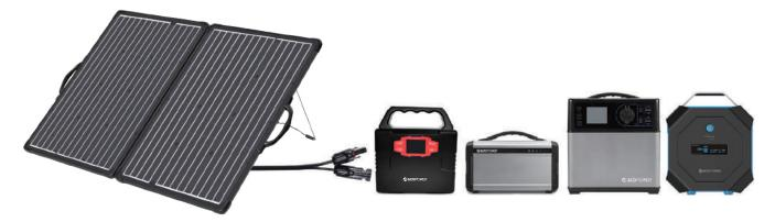
To test if the solar panel is working with a solar generator with a built-in charge controller, connect the MC4 adapters that came with your solar generator and plug it in to the MC4 cables of the solar panel directly (7a and 7b, Table 1). Turn your solar generator on and it should start charging from the solar panel.
