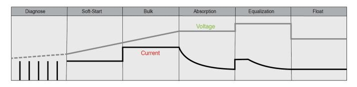
**Diagnose** \* – Only for Lithium battery type, subjected to the Lithium battery initial voltage then determinegoing to Soft start or Bulk charge; if the Lithium battery is protected by BMS, the controller will automatically send the sign al periodically to the battery terminal to activate the BMS against protection.
